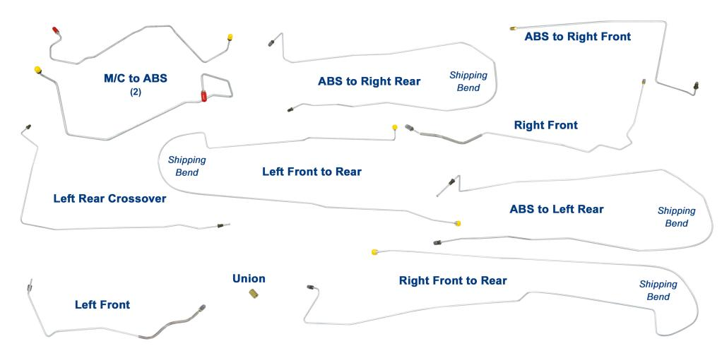
\*Re-designed for easier shipping/installation of factory brake lines for unmodified vehicles using original components.
