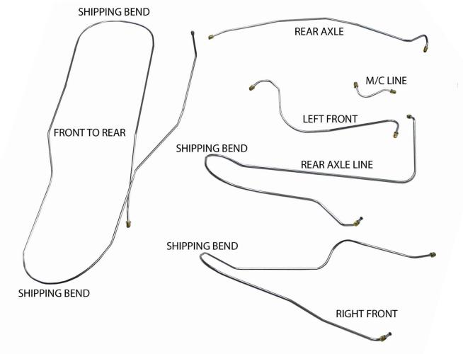
This is a factory brake line set for unmodified cars using original components.
