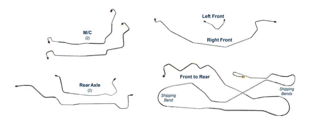
\*Reproduction of factory brake lines for unmodified vehicles using original components. Images are for identification purposes and are not to scale.
