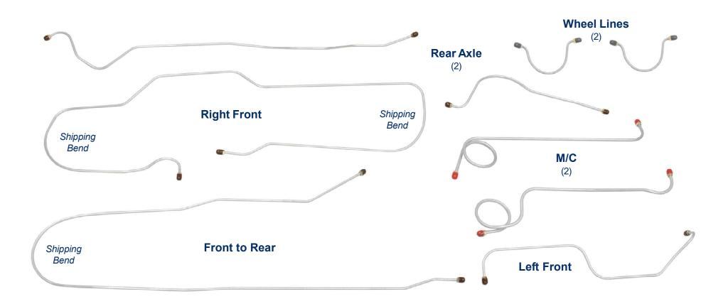
\*Reproduction of factory brake lines for unmodified vehicles using original components. Images are for identification purposes and are not to scale.
