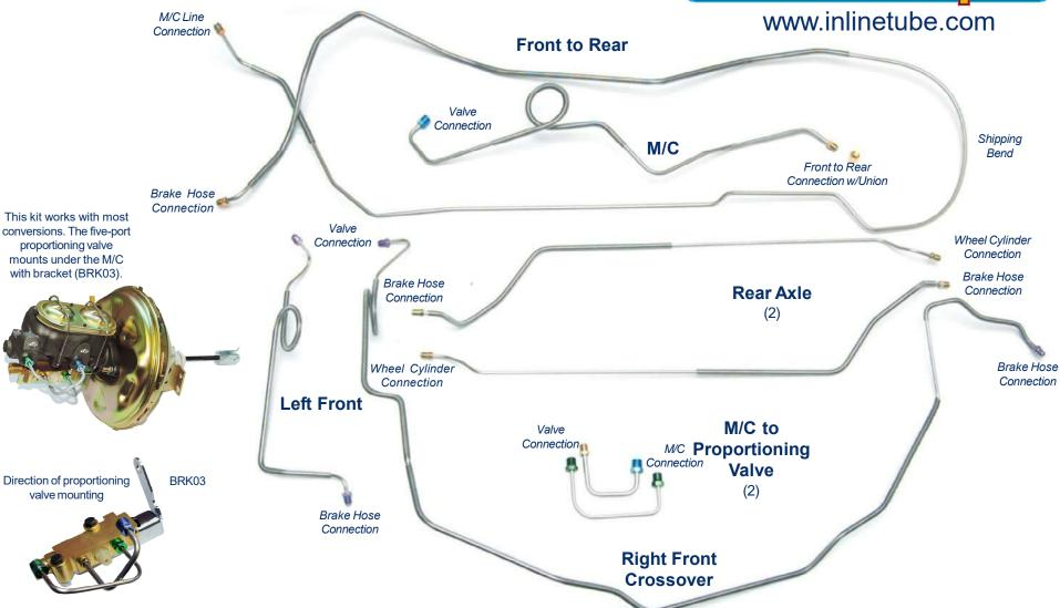
\*For vehicles converted to front disc with proportioning valve placement under M/C for clearance from frame and exhaust manifold.
