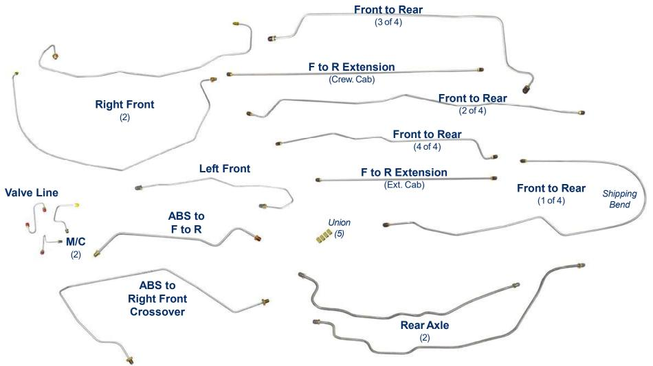
\*Re-designed for easier shipping/installation of factory brake lines for unmodified vehicles using original components. Specific applications may not require all pieces provided. Images are for identification purposes and are not to scale. © Inline Tube 2021
