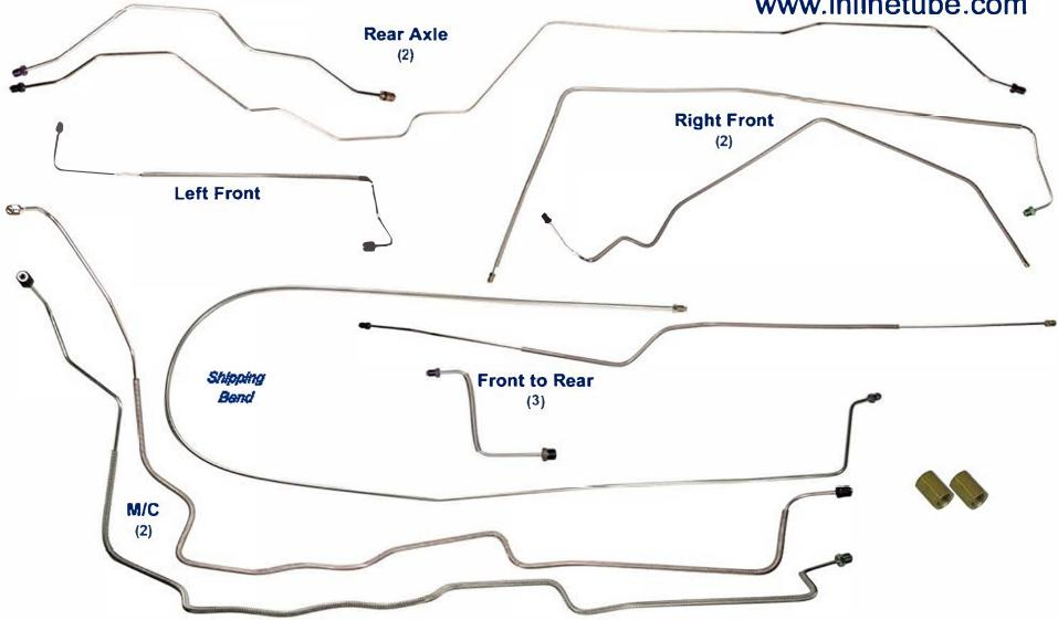
"Re-designed for easier shipping/installation of factory brake lines for unmodified vehicles using original components." Images are for identification purposes and are not to scale. ©Inline Tube 2023
