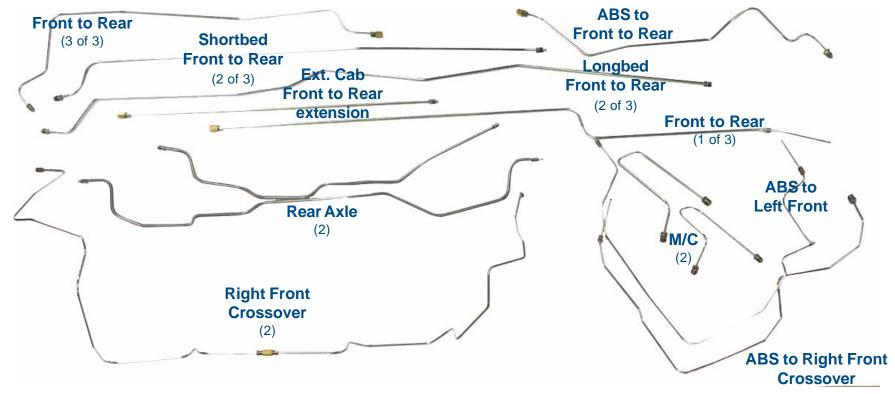
\*Re-designed for easier shipping/installation of factory brake lines for unmodified vehicles using original components. Specific applications may not require all pieces provided.
