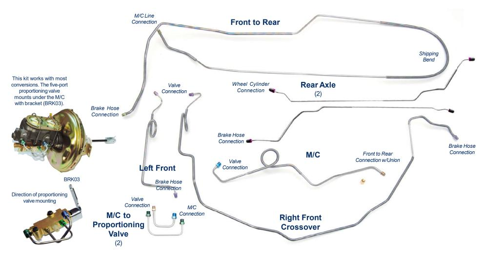
\*For vehicles converted to front disc with proportioning valve placement under M/C for clearance from frame and exhaust manifold. The correct proportioning valve bracket is Inline Tube part BRK03. Images are for identification purposes and are not to scale.
